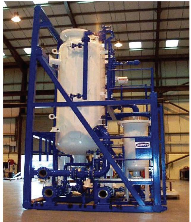
ToreSep - A compact bulk oil/water separator using vortex forces
